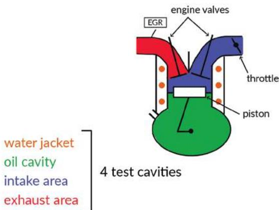
The classic engine air leak test cannot differentiate between a leak in the oil cavity, the intake or the exhaust since the parts are linked through the pistons rings. The rings are not completely leak tight because there is only a metal to metal contact between the piston rings and the cylinder.
