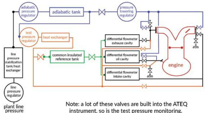
Note: a lot of these valves are built into the ATEQ instrument, so is the test pressure monitoring.
