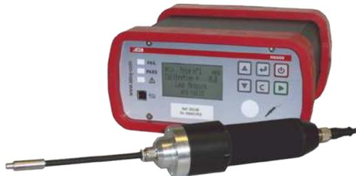
Getting an idea of where the leak is requires a bit more cycle time for air stabilization in the engine, but it can be achieved with a special ATEQ model MF differential flow tester.
