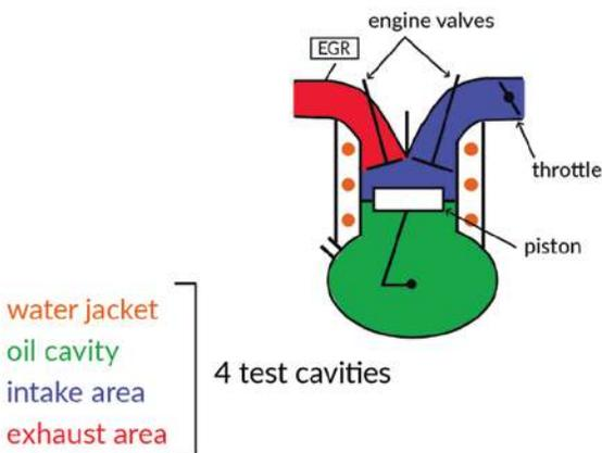
For example, if the engine valves were tested for leaks of maximum 100 sccm at 14.5 PSI, and the piston rings for 10,000 sccm at the same pressure, the maximum leak between two cavities would be the piston leak.
